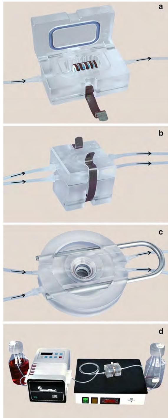
gradient perfusion culture container the tissue carrier is fixed centrally between the base and the lid. This design enables to transport different media at the luminal and basal side (Fig. 2b). For microscopic observation a
