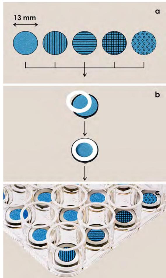
**Fig. 1** Application of a MINUSHEET<sup>®</sup> tissue carrier. **a** First a biomaterial measuring 13 mm in diameter is selected. **b** Then the biomaterial is placed in the black base part of a tissue carrier. Mounting is completed by pressing the white tension ring in the base part. **c** After sterilization the carrier is transferred by forceps to a 24 well culture plate for cell seeding
