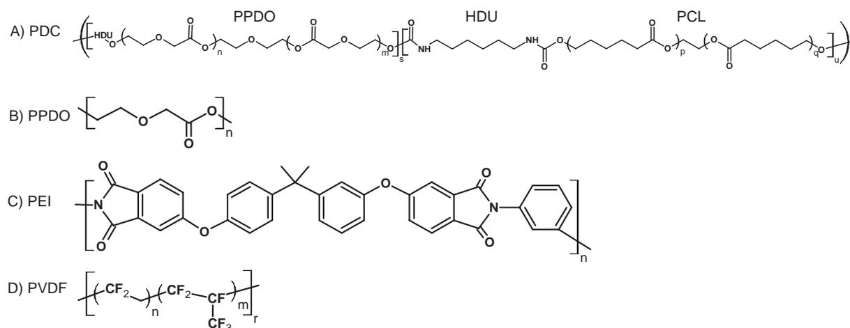
Fig. 1. Chemical structure of the polymers used for this study. (A) PDC, (B) PPDO, (C) PEI and (D) PVDF.
