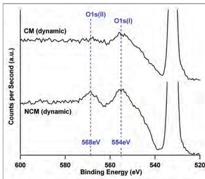
**Figure 5.** O1s loss spectrum of TCP-T ceramic after 8 d in NCM and CM culture media in dynamic conditions. The O1s photoelectric peak is located at 532 eV. The area ratio between the two components of the loss spectrum (554 eV and 568 eV) are modified by the culture conditions indicating a modification of the ceramic phases. The two spectra are represented with the same ordinate scale.
