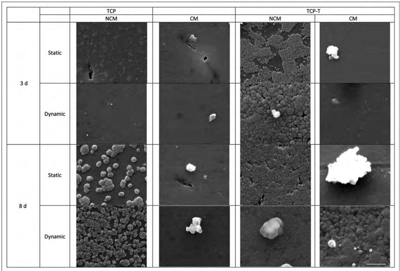
**Figure 4.** SEM micrographs of TCP and TCP-T samples after biomimetic study (bar = 5  $\mu\text{m}$ ).
