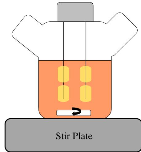
Fig. 1. Schematic of spinner flask bioreactor. Scaffolds are suspended in culture while media is circulated using a stir bar.
