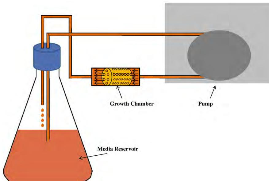
**Fig. 3.** Schematic of perfusion bioreactor. Media is directly perfused through porous scaffold sealed into a growth chamber.
