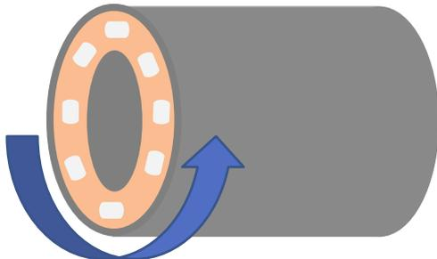
Fig. 2. Schematic of rotating wall bioreactor. Outside wall of bioreactor rotates to circulate media.
