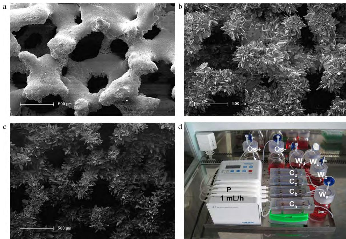
**Fig. 1.** (a) SEM-picture of unmodified iron foam (scale bar 500  $\mu\text{m}$ ); (b) SEM-picture of brushite-coated iron foam (scale bar 500  $\mu\text{m}$ ); (c) SEM-picture of HA-coated iron foam (scale bar 500  $\mu\text{m}$ ) and (d) perfusion culture: fresh basic medium ( $O_s^-$ ); fresh differentiation medium ( $O_s^+$ ); pump ( $P$ ) perfusion container ( $C_1$ – $C_4$ ), waste bottle ( $W_1$ – $W_4$ ).
