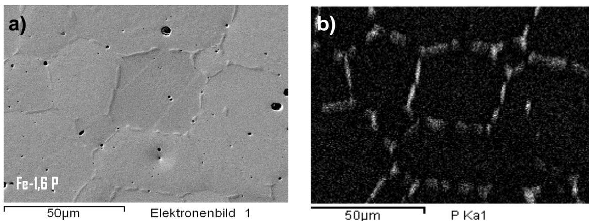
Figure 2: REM-picture (Figure a) and EDX-mapping of the Ka-line (Figure b) of pressed and sintered mixtures of carbonyl iron and 1.6 % phosphorus show a distinct phosphorus enrichment at the grain boundary.
