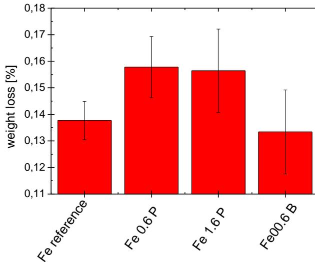
Figure 6: Degradation of pure iron, Fe-0.6P, Fe-1.6P, and Fe-0.06B.
