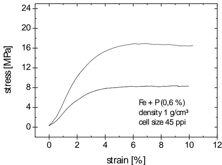
Figure 4: Compression-strain curves of a typical  $\text{Fe}_{0.6}\text{P}$  open cell metal foam with a density of  $1 \text{ g/cm}^3$ . The curves give the upper and the lower maximum of the compressive yield point. The medium compressive yield point is  $10.9 \pm 5.5 \text{ MPa}$ .
