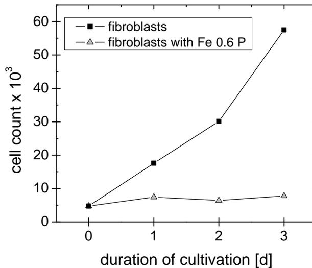
Figure 7: Cytotoxicity tests of fibroblasts in a dynamic perfusion chamber. Cells in contact to iron based alloys with 0.6 wt.-% phosphorus show a slight increase of the cell population.
