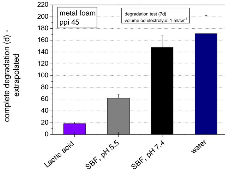
Figure 5: Degradation of iron foams in lactic acid, SBF and in water at 37 °C.
