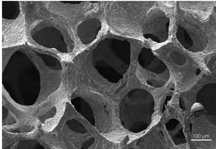
Figure 3. Electron microscopy picture of a metal foam made by a  $\text{Fe}_{0.6}\text{P}$  alloy.
