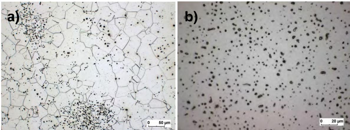
Figure 1: Metallographic cross sections of PM carbonyl iron samples with 0.6 wt.-% phosphorus (left side) and 0.06 % boron. In particular, the boron containing alloy show fine pores with a homogeneous distribution (right side).
