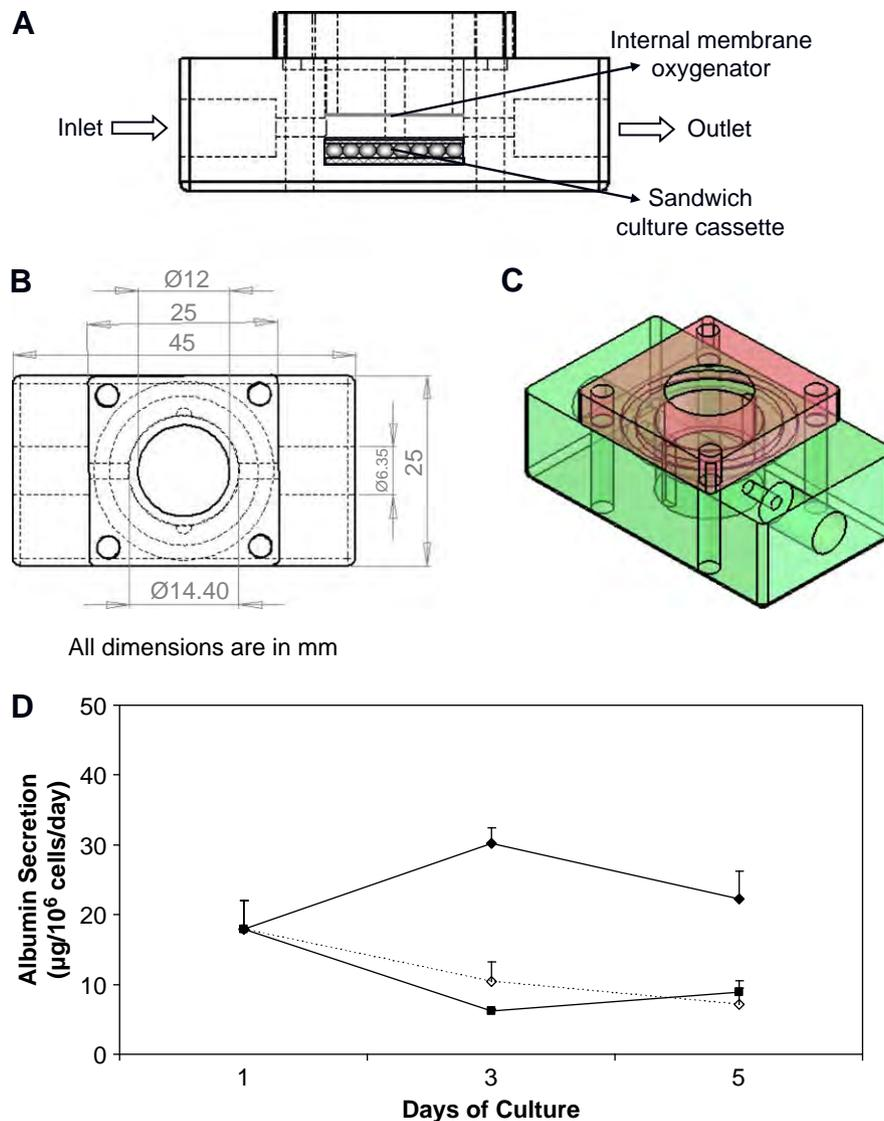
**Fig. 1.** Schematic of laminar-flow perfusion bioreactor. (A): Cross-sectional view; (B): top view, dimensions are in mm; (C): assembled bioreactor; (D): Influence of internal membrane oxygenator on the albumin secretion of hepatocytes. (◇) Static; (◆) perfusion with oxygenator; (■) perfusion without oxygenator.
