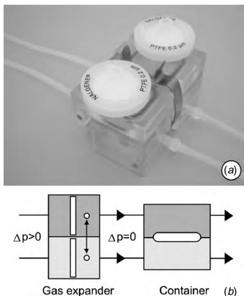
**Figure 7.** Use of a gas expander module in gradient perfusion culture. (a) Photograph shows the module with sterile filters attached to the ports at the top of the module. (b) The two individual channels of the module can be bridged to avoid pressure differences in the luminal and basal parts of the gradient perfusion culture container. Arrows indicate direction of flow.
