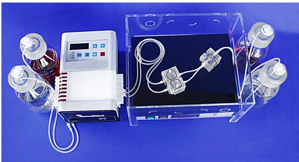
**Figure 3.** Perfusion culture setups are self-contained and can be used on a laboratory table. A peristaltic pump (left side) transports the media ( $1 \text{ ml h}^{-1}$ ) to a gas expander module and onward to a gradient container. The waste medium is collected in the bottles on the right side. A heating plate and a lid maintain the desired temperature.
