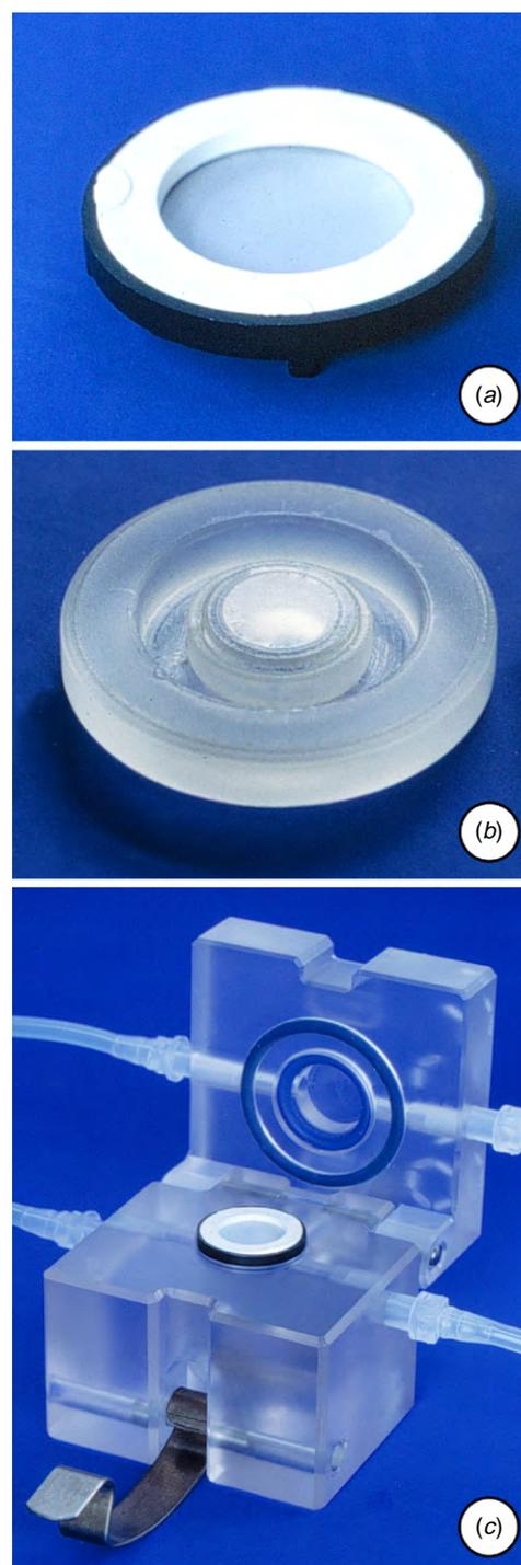
**Figure 2.** Illustration of different types of tissue carriers and a gradient culture container. (a) Inflexible materials such as filters with 13 mm diameter are placed in a holder and fixed by a tension ring. (b) Flexible matrices are held in place like the skin on a drum. (c) The gradient perfusion culture container consists of a basal and upper part. The tissue carrier is placed in the space between, thus dividing the two compartments.
