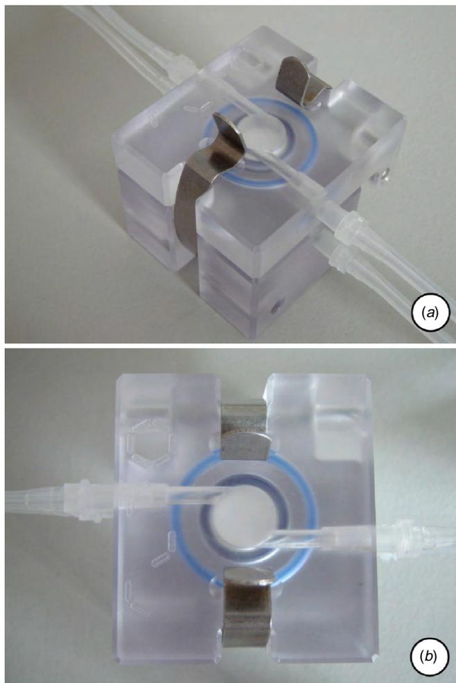
**Figure 9.** Photographs showing a redesigned gradient perfusion culture container. (a) Medium inlet and outlet are located at the tangential aspects of each tissue carrier. (b) When the gradient container is placed on its lateral side, medium enters now at the lowest point (right side), while the outlet (left side) is found at the highest point of the fluid reservoir. This innovative flow geometry leads to a continuous and efficient elimination of gas bubbles.
