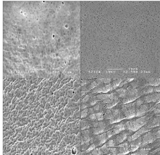
*Fig. 1: Effect of antibiotic sterilisation on flat sheet polymer morphology: control bottom (top left) control top (top right) sterilised bottom (bottom left) sterilised top (bottom right).*
