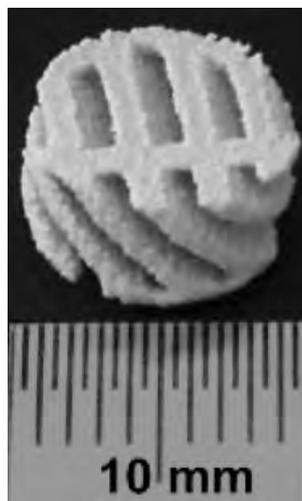
**Figure 3.** Printed test structure HA-S after sintering.
