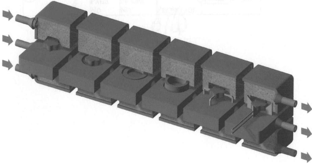
**FIG. 3.** Schematic representation of gradient perfusion containers with a basal plate and two lids each. The basal plate can house a variety of different tissue carriers with a diameter ranging between 13 and 47 mm.
