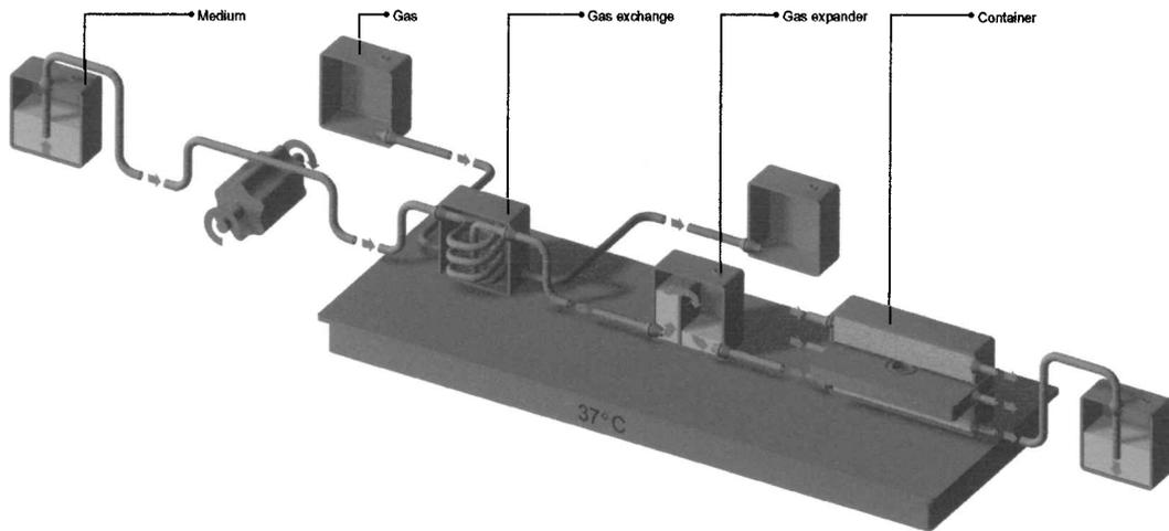
**FIG. 6.** Tissue Factory—a culture line for the generation of artificial tissue consists of a storage bottle for culture medium, a peristaltic pump, a gas exchanger, a gas expander to trap gas bubbles, a culture container, and a bottle to collect waste medium. The temperature of the whole system is maintained by a heating plate. Using a multichannel pump, several culture lines can be run in parallel.
