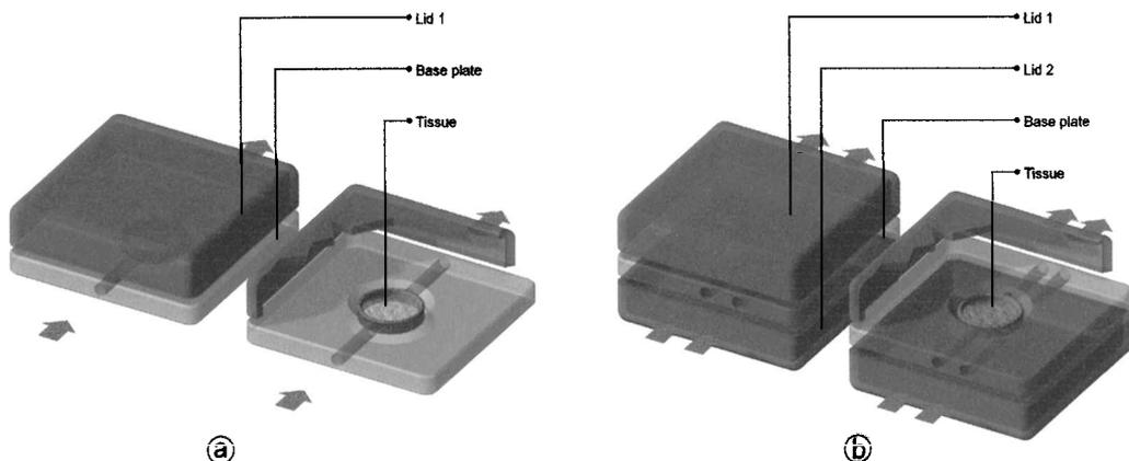
**FIG. 2.** Construction principle of culture containers with an artificial interstitium. (a) A perfusion container consists of a base plate to hold the developing tissue. The container is sealed with a lid filled with artificial interstitium. (b) A gradient perfusion container consists of a base plate with an opening for the developing tissue. Both sides of the plate are sealed with lids that contain artificial interstitium.
