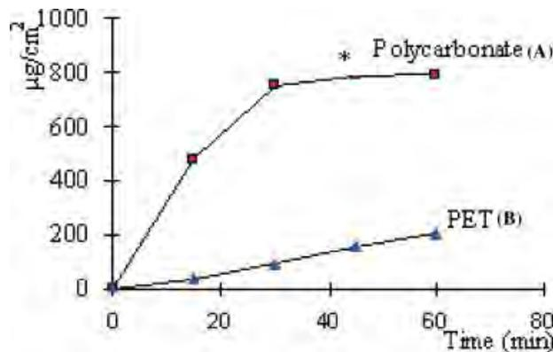
**Figure 6.** Schematic representation of the rate of theophylline transported through polycarbonate (A) or polyethylene terephthalate (B) support filters placed in Minucell rings free of cells. The experimental calculation is made with cumulative fraction of the drug transported. The results are plotted as µg/cm<sup>2</sup> in function of time and show statistically significant difference between polycarbonate and polyethylene terephthalate (*p* < 0.05).
