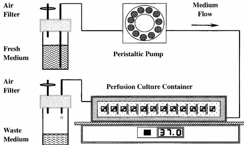
**FIG. 1.** Schematic diagram of the perfusion culture system. Block composites are held in a container through which fresh medium is delivered by a peristaltic pump at a rate of 2.0 mL/h. The container is maintained at 37°C by the thermo plate.
