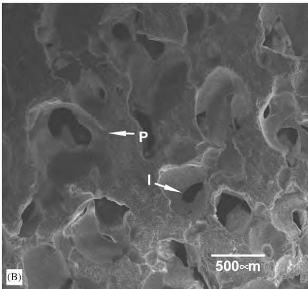
Fig. 4. SEM photomicrograph of microstructures of the novel porous hydroxyapatite (A) and beta-TCP(B). P indicates pore and I indicates interconnecting path.
