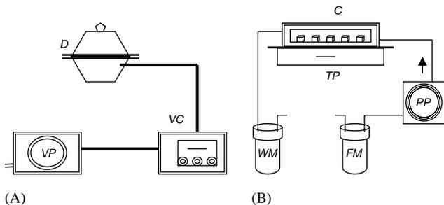
Fig. 3. Schematic diagram of the low-pressure system (A) and perfusion culture system (B). In (A), D stands for polycarbonate vacuum dessicator, and  $V_c$  for vacuum controller; in (B), C stands for perfusion container, TP for thermoplate, PP for peristaltic pump, FM for fresh medium, and WM for waste medium.
