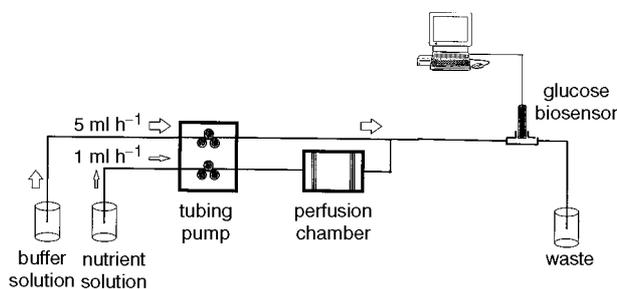
Fig. 1 Schematic setup of biosensor-controlled perfusion cell culture system
