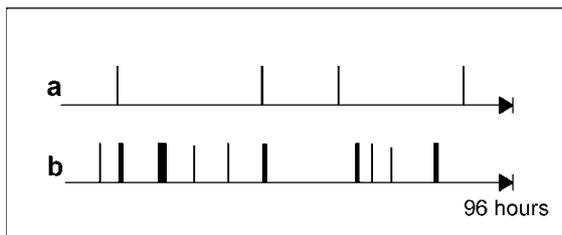
Fig. 4. Registration of gas bubbles passing through a gradient culture container by an infrared (IR) gate sensor over a 96 h period. The frequency and size of registered gas bubbles are indicated by black bars. It can be shown that the amount of gas bubbles is drastically decreased by the use of newly developed bottle closures and a gas expander module (a) as compared to controls without bubble elimination (b).
