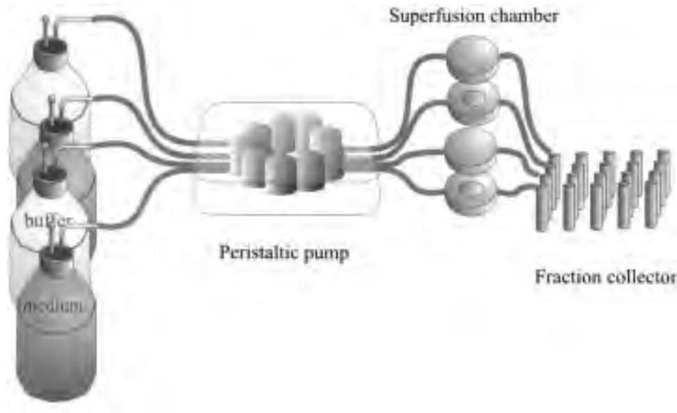
**Figure 2.** Set up of the superfusion system. A multi channel peristaltic pumps supplies incubation media to the superfusion chambers. The outflow is connected to a fraction collector, which collects the superfusate for further biochemical analysis.
