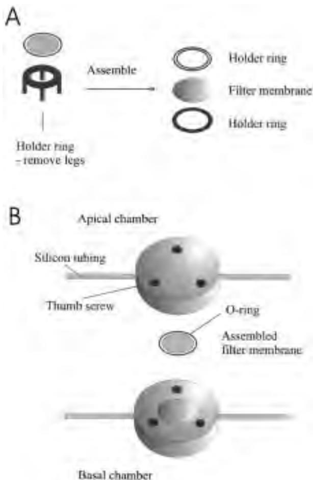
**Figure 1.** (A) Assembly of the filter membrane (Anodisc) and the Minusheet holder rings. The legs of the lower holder should be removed to assure a better sealing in the superfusion chamber. (B) The superfusion chamber basically is a modified Ussing chamber, in which the apical and the basal side of the filter membrane can be supplied with different incubation media. The tight sealing of the filter membrane within the experimental chamber is achieved by O-rings.
